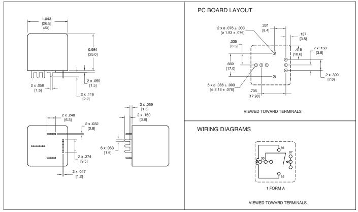
Dimensions in inches with millimeters in brackets below. Tolerance:  $\pm .010$ "
