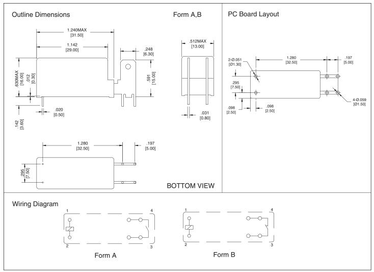
Dimensions in inch with millimeters in brackets below. Tolerance: ± .010"
