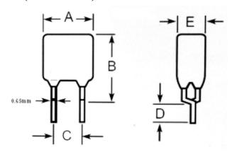
Lead Size: 22AWG 0.65 mm Diameter
