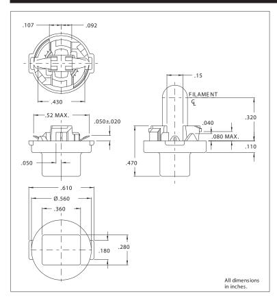
Mounting: Printed circuit board, twist-in
