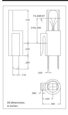
Mounting: Snap-on edge or center Mounting pattern on page SP1. Terminals: Tinned brass Housing: White nylon Lamp: T-1 3/4 Wedge base Note: Lamps must be ordered separately.
