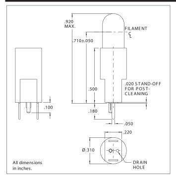
Mounting: Press-in mounting for accurate location on printed circuit board.
