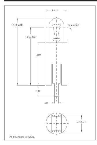
Mounting: Printed circuit Board
