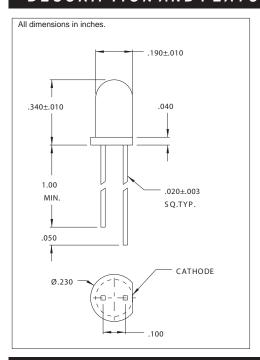
These white diffused with pale tint LED lamps provide maximum on/off contrast in high ambient lighting levels. These lamps are designed with wide view angles for direct viewing. The High Efficiency Red/Orange and Yellow lamps are produced with GaAsP/GaP, the High Efficiency Green lamps are produced with GaP/GaP and the red (dark red) lamps are produced with AlGaAs.
