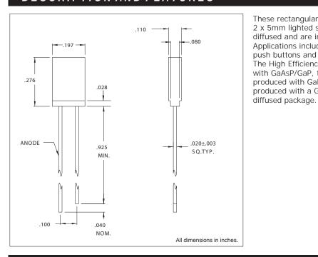
These rectangular LED lamps with flanges provide a 2 x 5mm lighted surface area. Lamps are tinted diffused and are intended for direct viewing. Applications include legend backlighting, illuminated push buttons and panel indicators. The High Efficiency Red and Yellow lamps are produced with GaAsP/GaP, the High Efficiency Green lamp is produced with GaP/GaP, and the Orange lamp is produced with a GaAsP/GaP chip in an orange tinted
