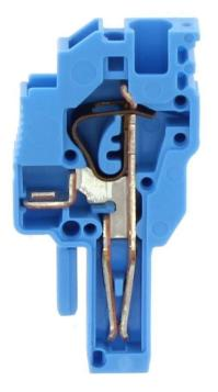
Feed-through terminal, Tension-spring connection, Mounting type: Plug in, Rated cross-section: 2.5 mm<sup>2</sup>, Width: 5.1 mm, Colour: Blue
