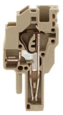
Feed-through terminal, Tension-spring connection, Mounting type: Plug in, Rated cross-section: 2.5 mm<sup>2</sup>, Width: 5.1 mm, Colour: Beige
