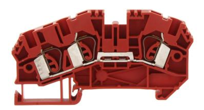
Feed-through terminal, Tension-spring connection, Mounting type: Mounting rail TS 35/7.5, Rated cross-section: 4 mm², Width: 6.1 mm, Colour: Red
