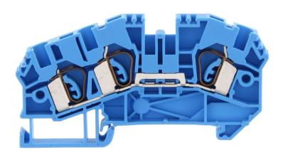
Feed-through terminal, Tension-spring connection, Mounting type: Mounting rail TS 35/7.5, Rated cross-section: 4 mm², Width: 6.1 mm, Colour: Blue
