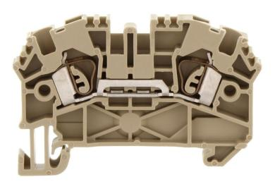
Feed-through terminal, Tension-spring connection, Mounting type: Mounting rail TS 35/7.5, Rated cross-section: 2.5 mm², Width: 5.1 mm, Colour: Beige
