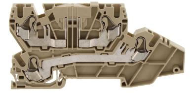
Three-wire installation terminal, Push-in connection, Mounting type: Mounting rail TS 35/7.5, Rated cross-section: 4 mm<sup>2</sup>, Width: 5.1 mm, Colour: Beige
