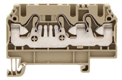
Feed-through terminal, Push-in connection, Mounting type: Mounting rail TS 35/7.5, Rated cross-section: 4 mm<sup>2</sup>, Width: 6.1 mm, Colour: Beige
