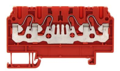
Feed-through terminal, Push-in connection, Mounting type: Mounting rail TS 35/7.5, Rated cross-section: 1.5 mm², Width: 4.1 mm, Colour: Red
