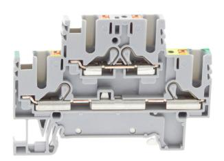
Double-level terminal, Push-in connection, Mounting type: Mounting rail TS 35/7.5, Rated cross-section: 2.5 mm², Width: 5.1 mm, Colour: Grey
