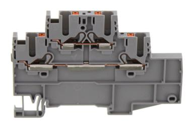
Three-level initiator terminal |Multi-wire terminal, Push-in connection, Mounting type: Mounting rail TS 35/7.5, Rated cross-section: 2.5 mm², Width: 5.1 mm, Colour: Grey
