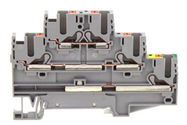
Three-level initiator terminal |Multi-wire terminal, Push-in connection, Mounting type: Mounting rail TS 35/7.5, Rated cross-section: 2.5 mm², Width: 5.1 mm, Colour: Grey
