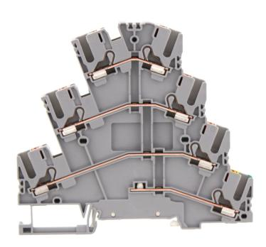
Three-level initiator terminal |Multi-wire terminal, Push-in connection, Mounting type: Mounting rail TS 35/7.5, Rated cross-section: 2.5 mm², Width: 5.1 mm, Colour: Grey
