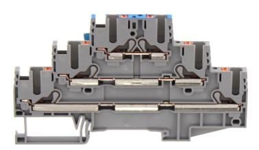
Three-level initiator terminal |Multi-wire terminal, Push-in connection, Mounting type: Mounting rail TS 35/7.5, Rated cross-section: 2.5 mm², Width: 5.1 mm, Colour: Grey
