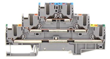
Three-level initiator terminal |Multi-wire terminal, Push-in connection, Mounting type: Mounting rail TS 35/7.5, Rated cross-section: 2.5 mm<sup>2</sup>, Width: 5.1 mm, Colour: Grey
