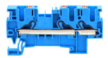
Feed-through terminal, Push-in connection, Mounting type: Mounting rail TS 35/7.5, Rated cross-section: 4 mm², Width: 6.1 mm, Colour: Blue
