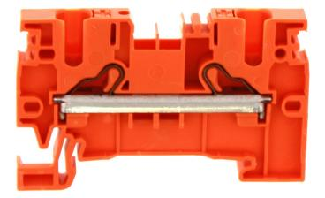
Feed-through terminal, Push-in connection, Mounting type: Mounting rail TS 35/7.5, Rated cross-section: 4 mm<sup>2</sup>, Width: 6.1 mm, Colour: Orange
