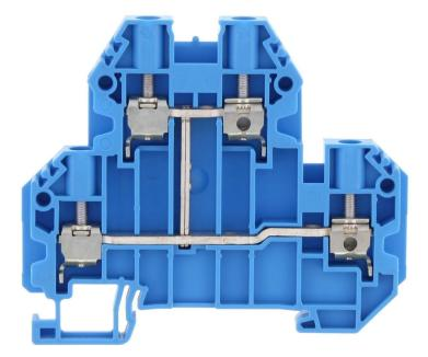
Double-level terminal, Screw connection, Mounting type: Mounting rail TS 35/7.5, Rated cross-section: 4 mm<sup>2</sup>, Width: 6.1 mm, Colour: Blue
