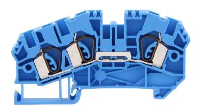
Ex feed-through terminal ATEX-certified, Tension-spring connection, Mounting type: Mounting rail TS 35/7.5, Rated cross-section: 4 mm², Width: 6.1 mm, Colour: Blue
