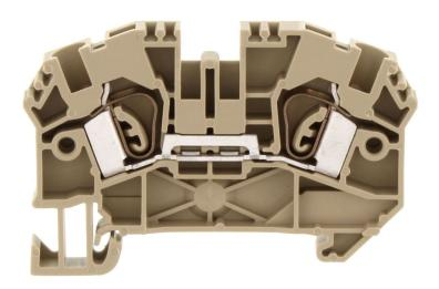
Ex feed-through terminal ATEX-certified, Tension-spring connection, Mounting type: Mounting rail TS 35/7.5, Rated cross-section: 4 mm², Width: 6.1 mm, Colour: Beige
