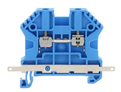
Feed-through terminal, Screw connection, Mounting type: Mounting rail TS 35/7.5, Rated cross-section: 2.5 mm², Width: 5 mm, Colour: Blue
