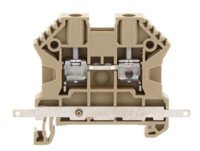
Feed-through terminal, Screw connection, Mounting type: Mounting rail TS 35/7.5, Rated cross-section: 4 mm², Width: 6 mm, Colour: Grey
