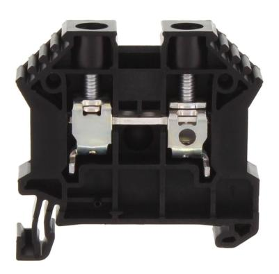
Feed-through terminal, Screw connection, Mounting type: Mounting rail TS 35/7.5, Rated cross-section: 16 mm², Width: 10 mm, Colour: Black
