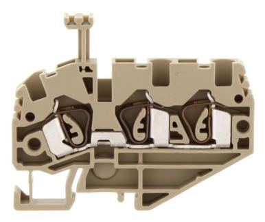
Ex feed-through terminal ATEX-certified, Tension-spring connection, Mounting type: Mounting rail TS 15/5.5, Rated cross-section: 2.5 mm<sup>2</sup>, Width: 5.1 mm, Colour: Beige
