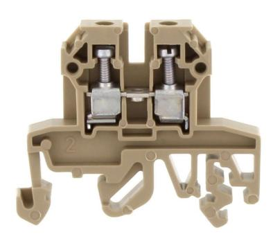
Feed-through terminal, Screw connection, Mounting type:Mounting rail TS 35/7.5 and TS 32, Rated cross-section: 2.5 mm², Width: 5 mm, Colour: Beige
