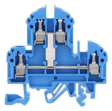
Double-level terminal, Screw connection, Mounting type:Mounting rail TS 35/7.5 and TS 32, Rated cross-section: 4 mm<sup>2</sup>, Width: 6 mm, Colour: Blue
