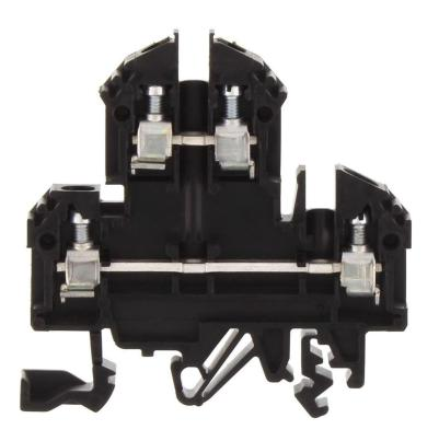
Double-level terminal, Screw connection, Mounting type:Mounting rail TS 35/7.5 and TS 32, Rated cross-section: 4 mm², Width: 6 mm, Colour: Black
