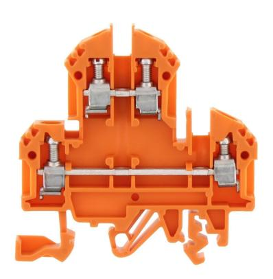
Double-level terminal, Screw connection, Mounting type:Mounting rail TS 35/7.5 and TS 32, Rated cross-section: 4 mm², Width: 6 mm, Colour: Orange
