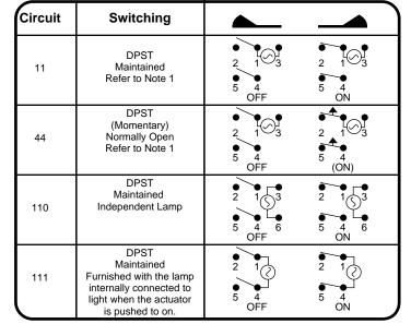
NOTE 1. Furnished with one side of the lamp internally connected and a single lamp-terminal at the back of the switch.
