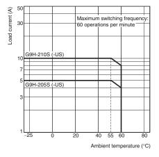
Lamp load (Inrush current: 6 times the rated current, Inrush current time: 2 cycles
