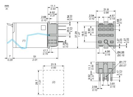
(1) : (2) : Metal hold-down clip Recommended chassis cutout top view Connections and Schema
