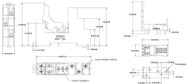
Tolerances: ± 0.02 in / 0.5 mm. All dimensions are in: inches [millimeters]
