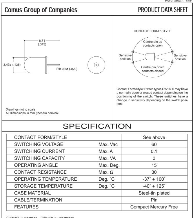
CW1600-0 I electrode CW1600-3 2 electrodes
